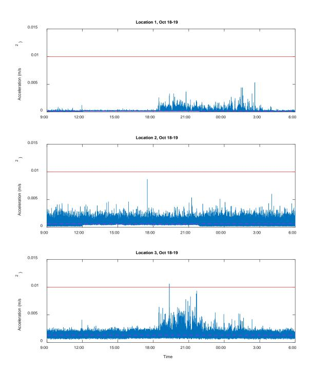
Figure 1: RMS particle accelerations at Location 1, 2 and 3 on October 18-19, 2017. The magenta dash line represents the mean baseline rms particle acceleration calculated from October 5 to 16 at each location. The red line shows the 0.01 m/s<sup>2</sup> threshold of the RMS particle acceleration.
